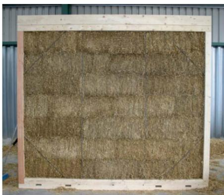
Constructed with the load-bearing straw panels within an airtight design (plus triple glazed windows) the new houses will need significantly less conventional heating. Their super-insulated straw walls provide three times' greater insulation than required by current UK building regulations so fuel bills are anticipated to fall by up to 90%.
